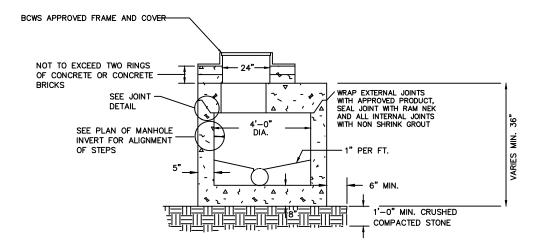
NOTE: FLAT TOP MANHOLE FRAME AND COVER MAY BE REQUIRED FOR SHALLOWER INSTALLATION PENDING BCWS APPROVAL
